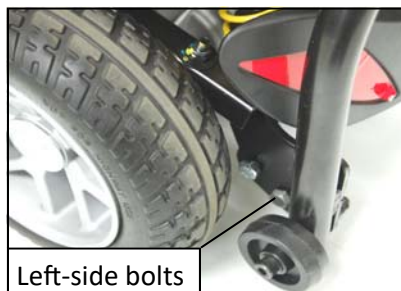
Figure 2: Rear Bumper Installed
